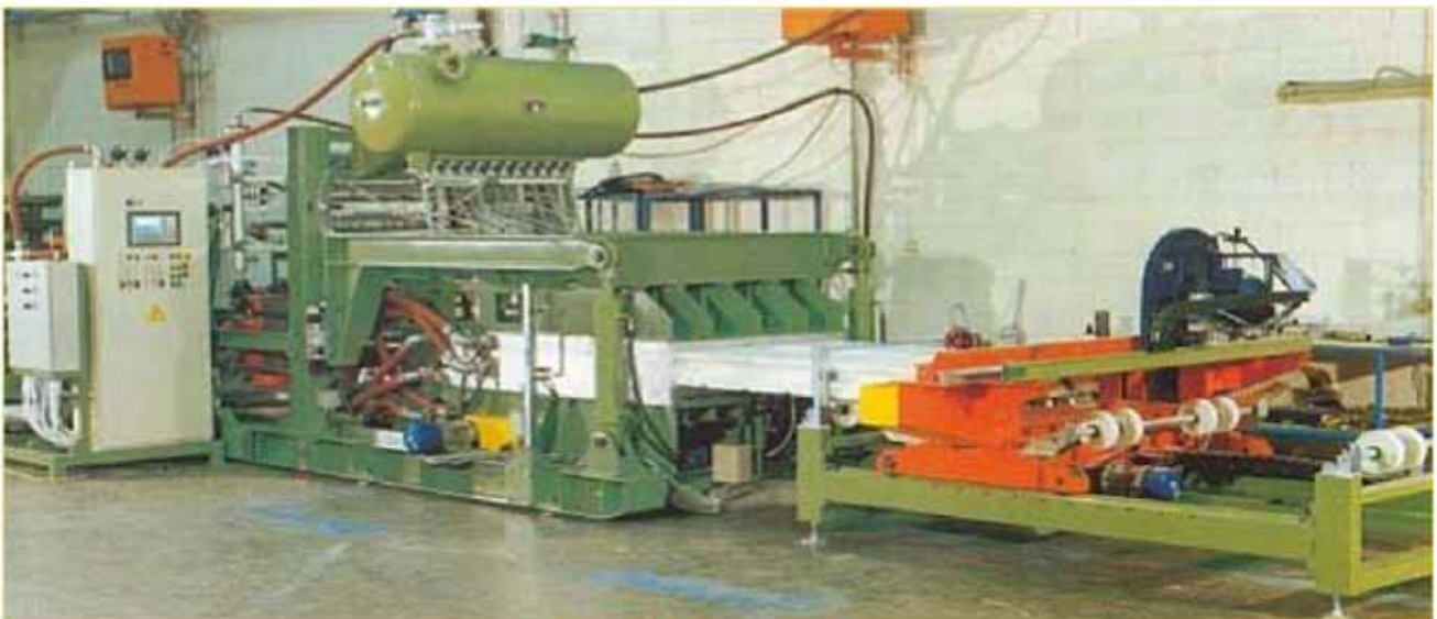
Continuous forming machine for PLASTBAU® METAL panels; production rate: (40-50 m 2 / h)
